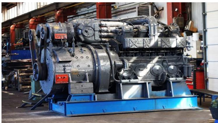
*Figure 2.* A8C22 internal combustion engine.
