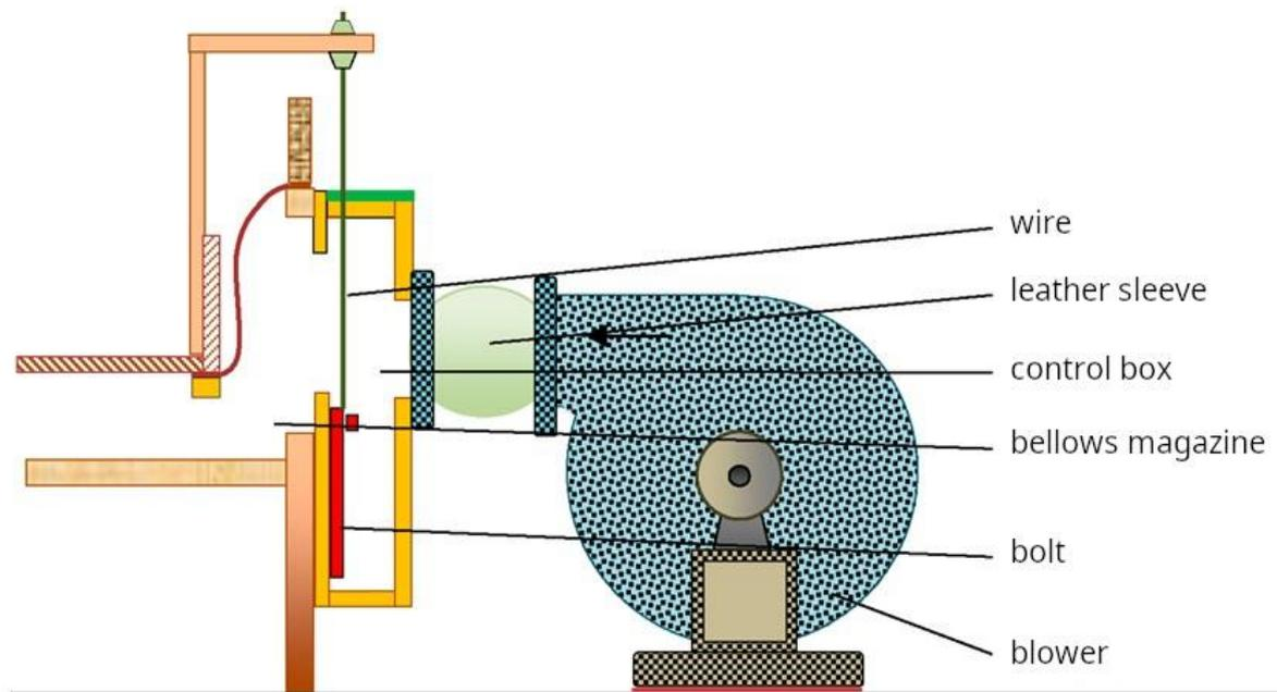
Figure 1. Organ blower including a damper that closes off air access to the bellows.
