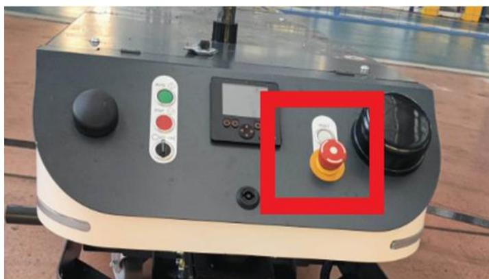
*Figure 10.* Main safety switch on the AGV (technological audit).
