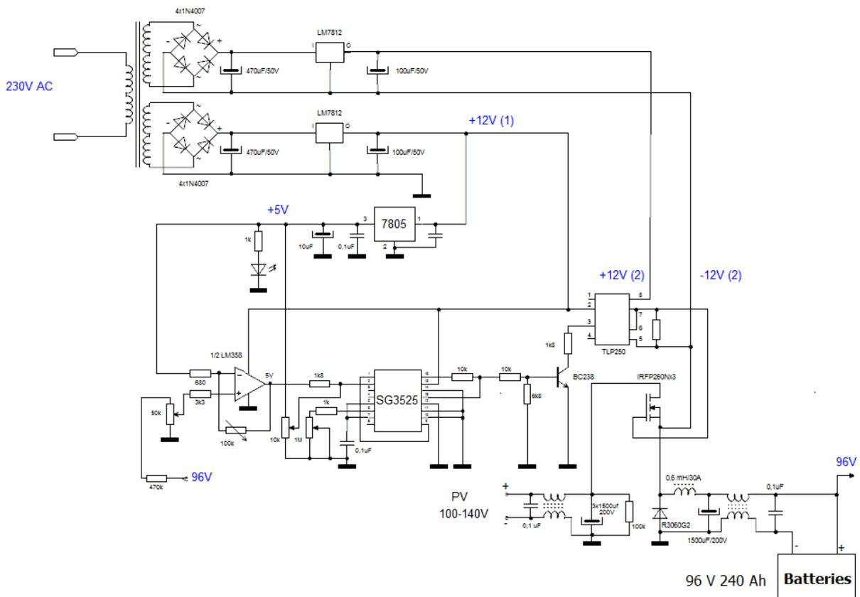
*Figure 4.* Schematic diagram of a pulse charge regulator.
