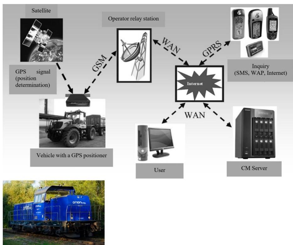
Figure 1. Block layout of the GPS monitoring system.
