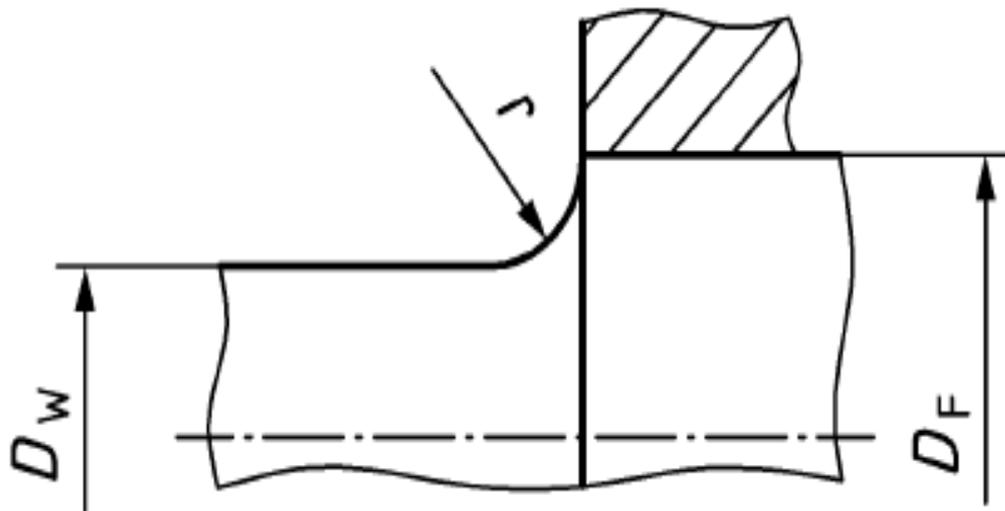
Figure 1. Optimized transition between different diameters (DIN 7190-1:2017-02).
