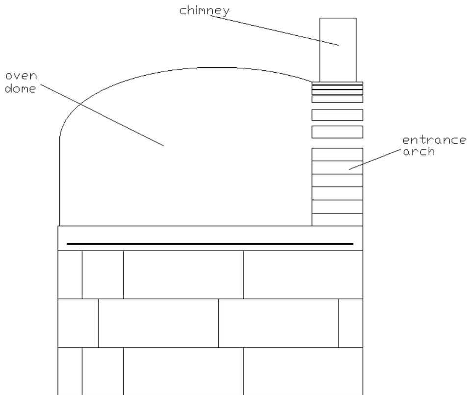
*Figure 3.* Side view of the oven.
