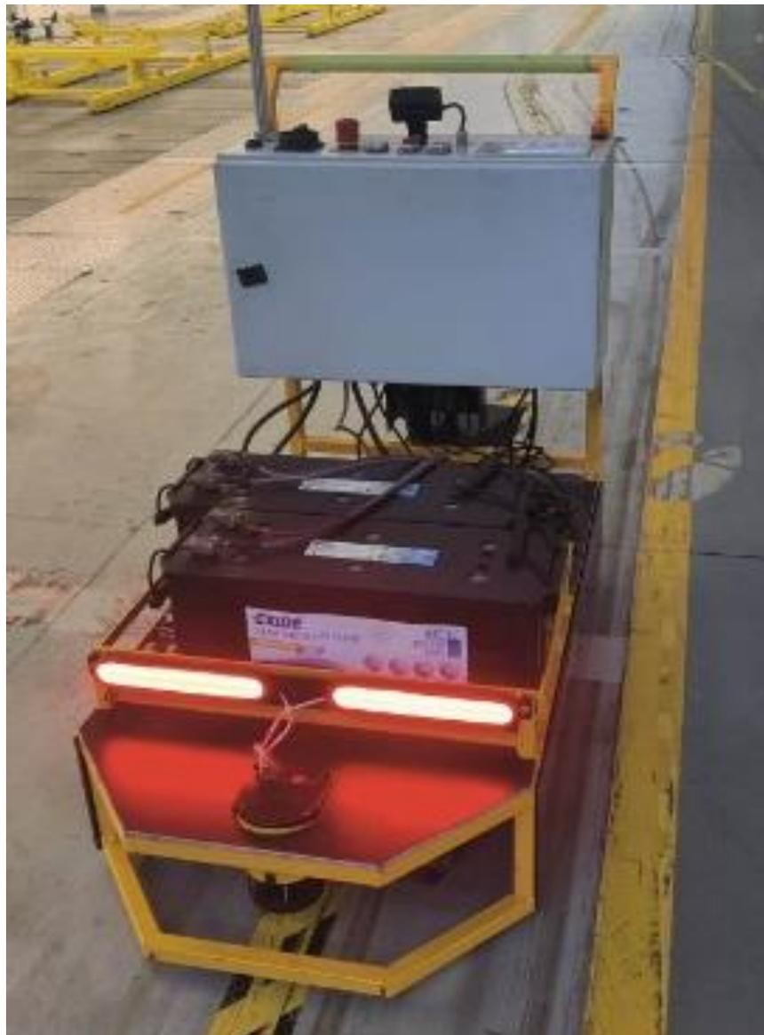
*Figure 11.* Traffic lights showing the status of the AGV (technological audit).
