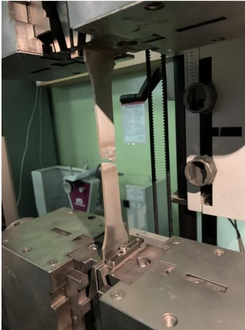
*Figure 5. Sample mounted on Zwick/Roell Z 100 ripper. View after rupture.*
