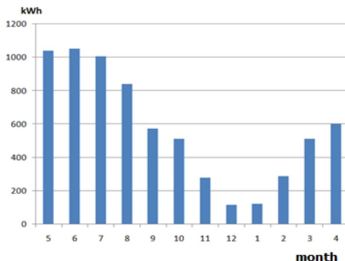
Figure 6. Energy produced in the prosumer system during the year (in the months: from May to April).
