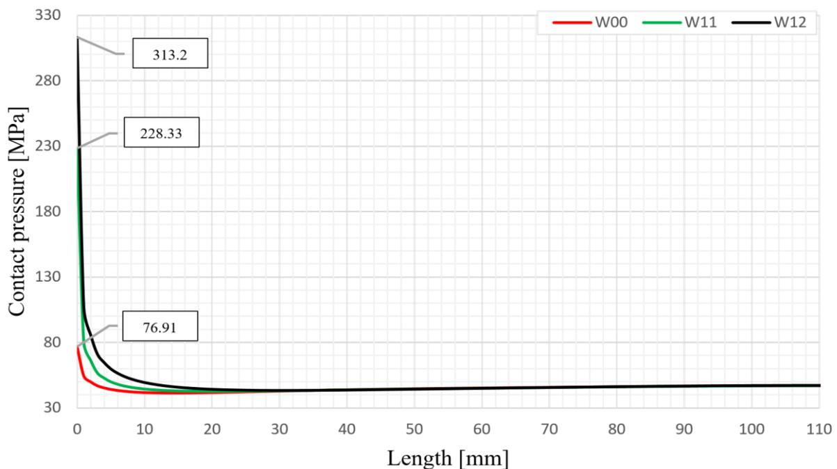
Figure 10. Distribution of contact pressure along an interference fit connection. Variants W00, W11, W12.
