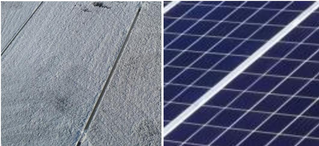
*Figure 12.* View of the module surface covered with snow after partial (left) and complete snow removal (right).
