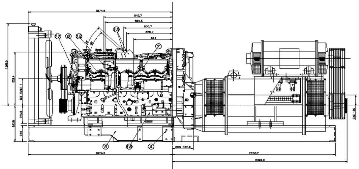
Figure 8. Diagram of the power generator of the modernized 6Dm locomotive.
