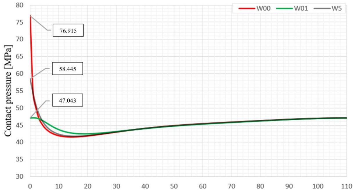
Figure 9. Distribution of contact pressure along an interference fit connection. Variants W00, W01, W5.
