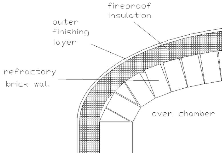
*Figure 5.* Cross-section of the oven wall.
