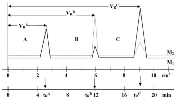
Figure 2. The process of creating a chromatogram.
