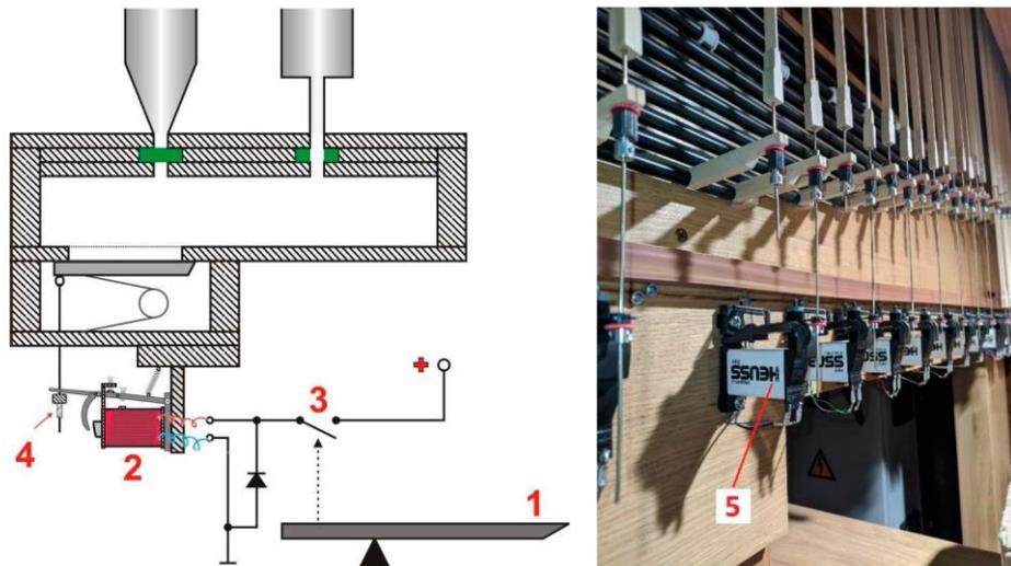
Figure 2. Electromagnetic tractive mechanism of play.
