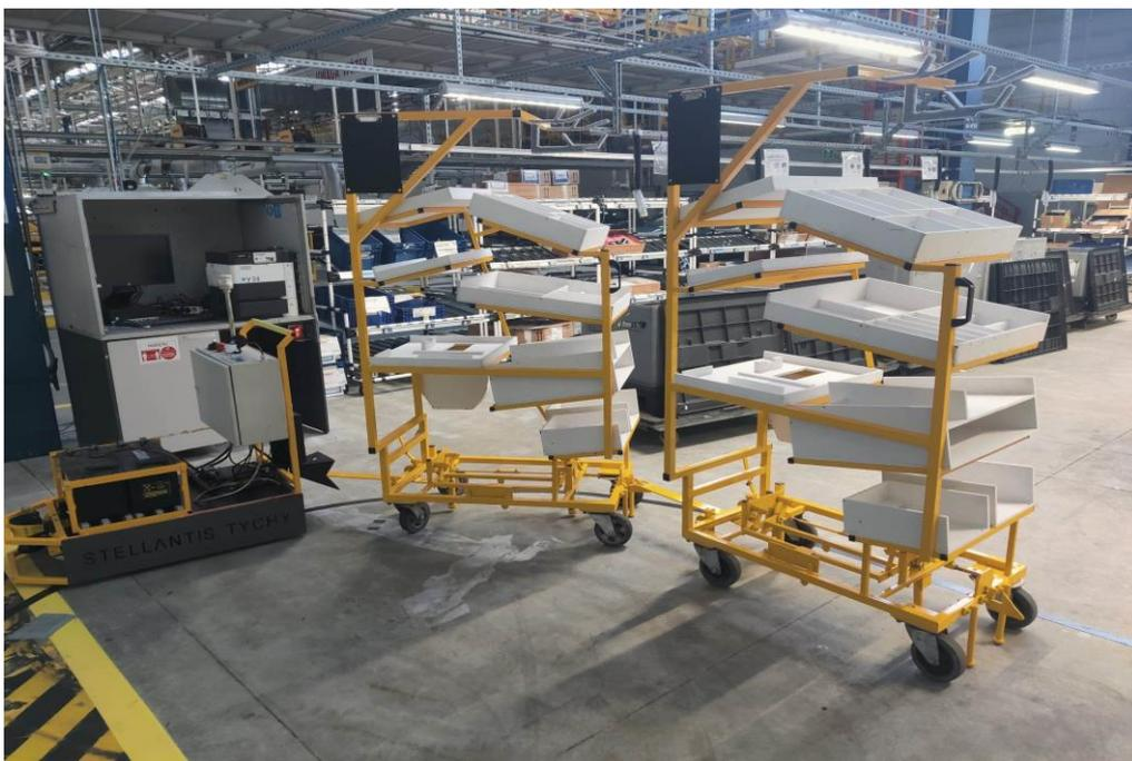
*Figure 8.* AGV trolley with trolleys transporting small assembly elements (technological audit).
