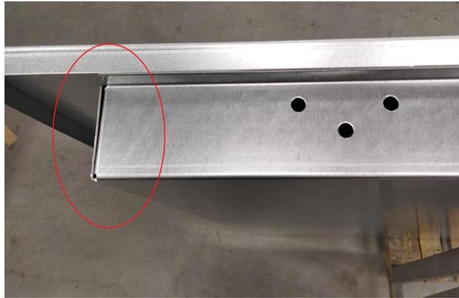
Figure 3. Badly dogged angle of inner plating.
