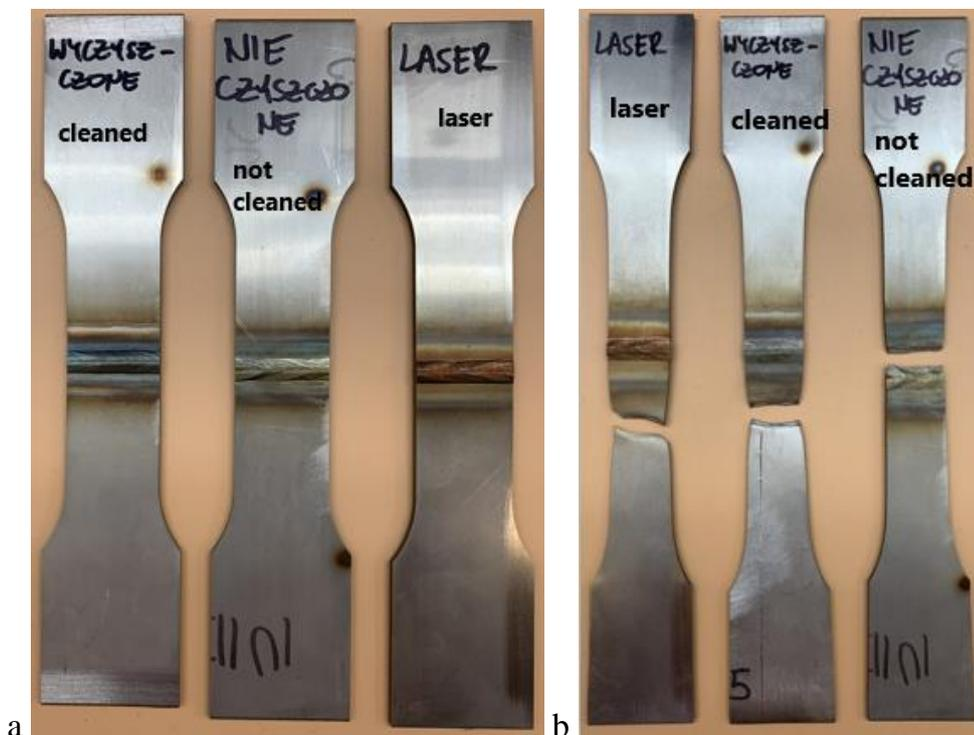
Figure 4. Views of samples used in static tensile testing, (a) pre-rupture view of samples, (b) post-rupture view of samples. Source: own elaboration.
