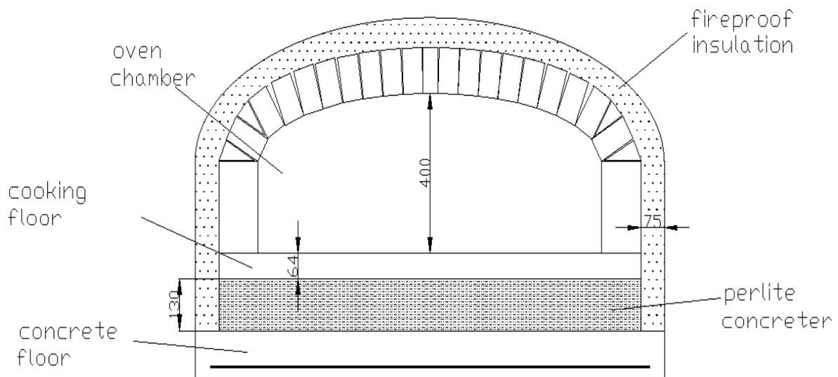
*Figure 4.* The shape of the oven chamber.
