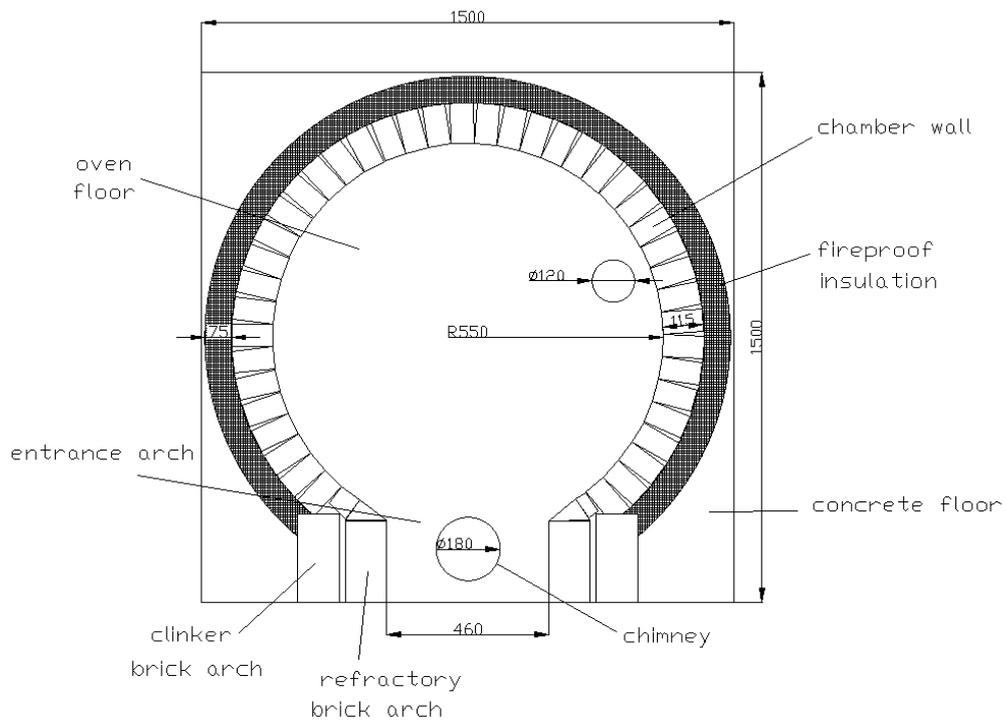
*Figure 2.* Top view of the oven.
