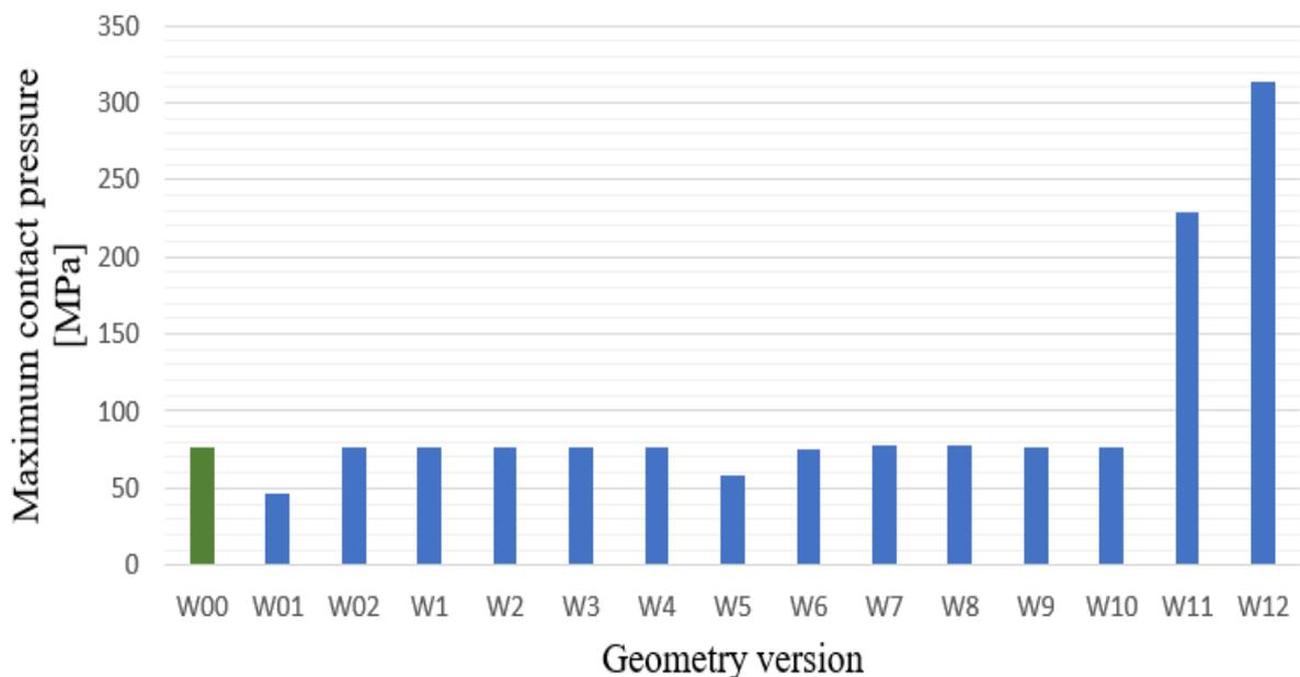
Figure 8. Maximum contact pressure for all variants.
