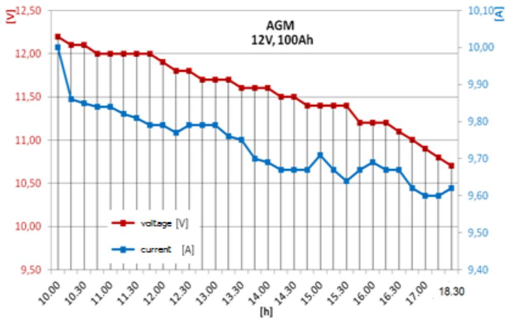
Figure 9. Battery voltage and discharge current characteristics for T = +50°C.
