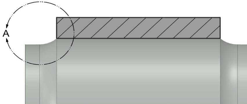
Figure 3. Cross section of the analyzed interference fit.
