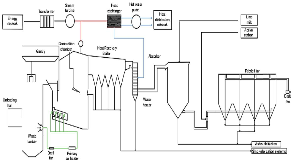
Figure 10. Technological scheme of the plant for thermal treatment of waste.
