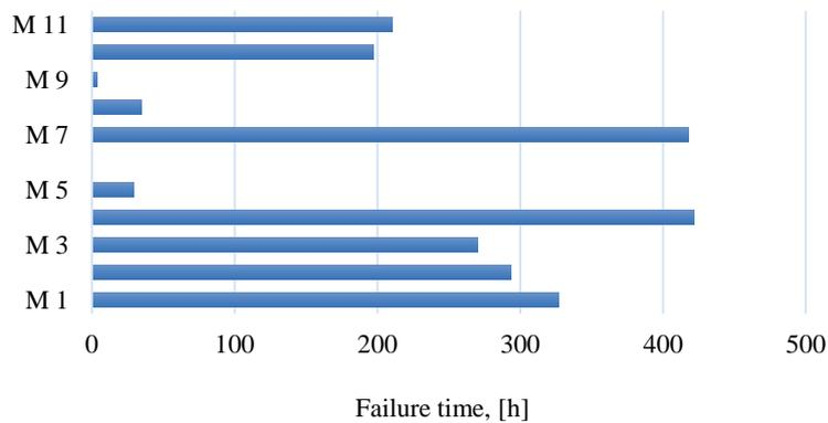
Figure 1. Total downtime due to individual machine failures.
