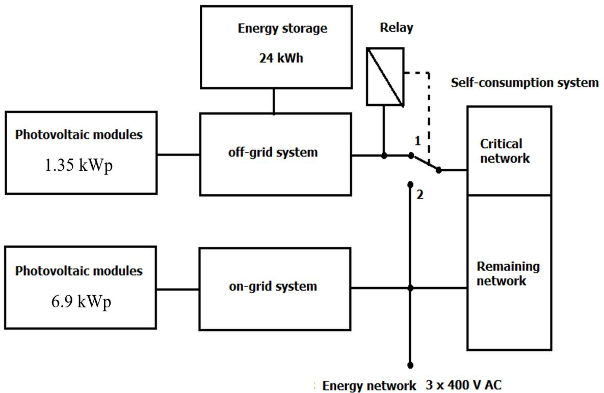
Figure 1. The concept of a complementary energy system.
