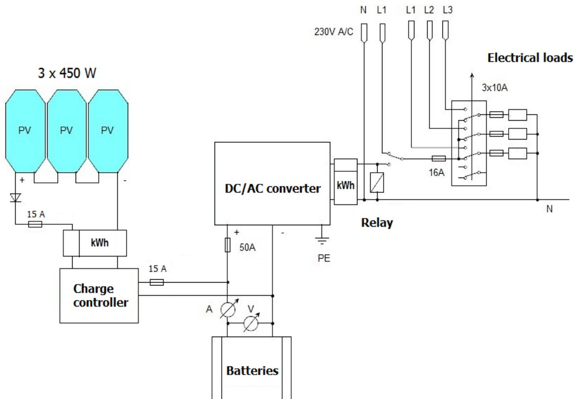
*Figure 3.* Block diagram of the off-grid system.
