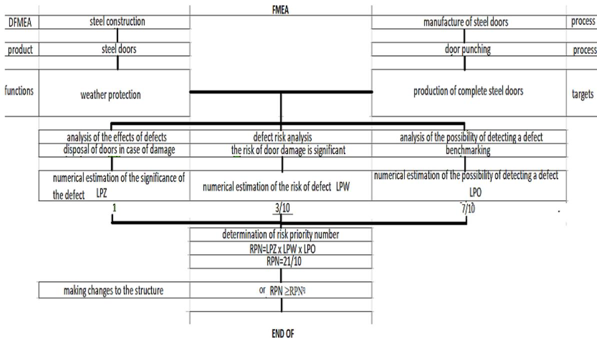
Figure 5. Algorithm of FMEA method of construction.
