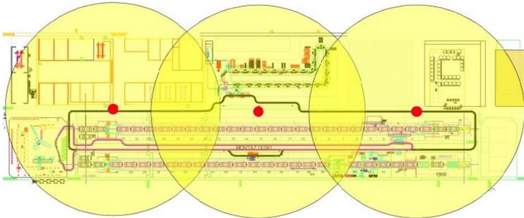
*Figure 7.* Location of wireless network access points within the car assembly hall.
