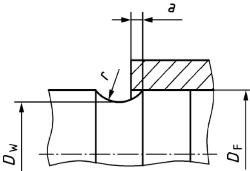
Figure 2. Example of optimizing the transition by undercutting the journal and projecting the hub (DIN 7190-1:2017-02).
